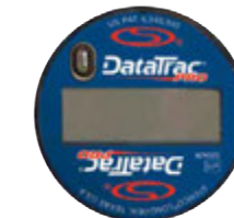
Display turns off when vibration is detected (vehicle moving) to conserve energy.
