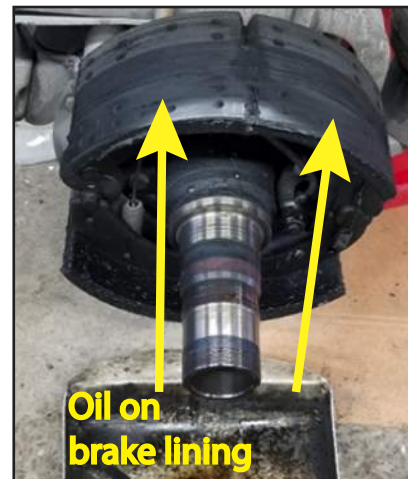
Figure 12: Leaking Seal - Drum Brake Active Oil Contamination on Brake Lining
