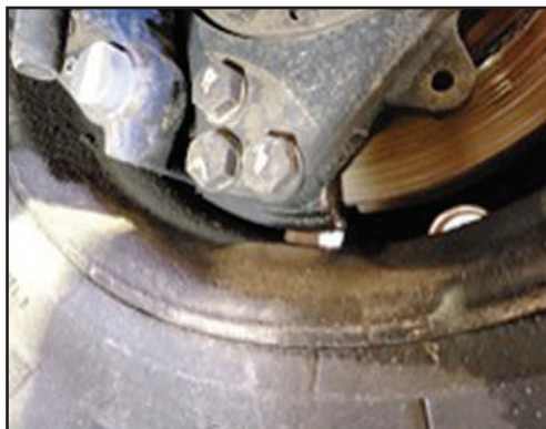
Figure 10: Weeping Seal — Disc Brake Requires Monitoring
