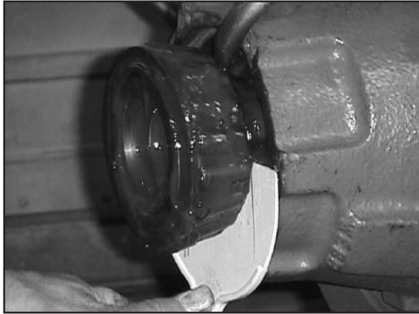
Fig. 5C: Using Template to Hold Lubricant
