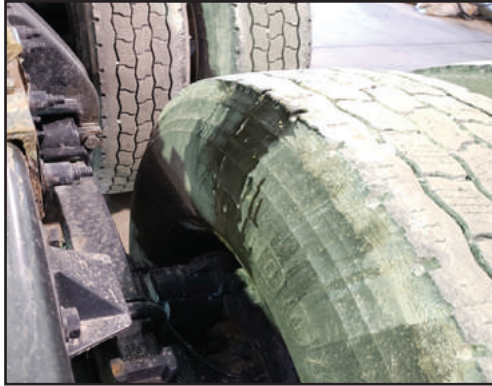
Figure 13: Oil Staining on Tires — Leaking Seal; Disc Brake
