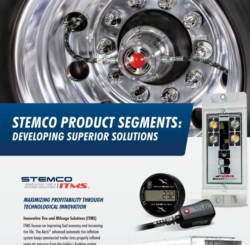
ITMS focuses on improving fuel economy and increasing tire life. The Aeris® advanced automatic tire inflation system keeps commercial trailer tires properly inflated using air pressure from the trailer's braking system.
