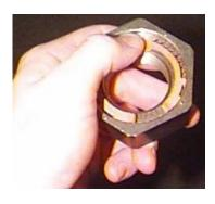
Place the blade of a flat-head screwdriver in the slot located on the keeper leg.
