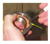
**DO NOT** place the blade of the screwdriver in any other location along the keeper leg.
