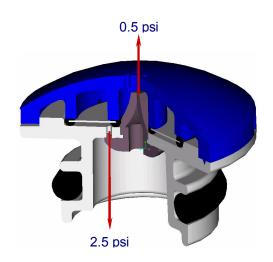
into the Sentinel system as part of its contaminant exclusion function. It is present for both the Sentinel Hub Cap and the ESP. Please note that this vacuum does not affect seal performance for three primary reasons:
