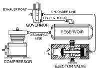
FIGURE 3 COMPRESSOR CUTTING "OUT"
