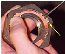
4. Pry the keeper leg until it is out of the nut groove.
