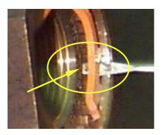
3. Work the blade of the screwdriver past the keeper leg, until it is in contact with the nut. This can be accomplished by prying on the screwdriver while moving it back and forth. Make sure the blade is in contact with the surface (as shown below), not the nut teeth.
