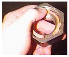
1. Hold the ProTorq nut assembly firmly in one hand. Locate the thumb over the tab/Dflat feature.
