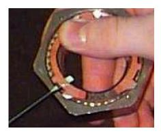
5. Change hands and repeat to remove the other keeper leg. Be sure to hold the keeper firmly with the thumb. This will prevent the keeper from springing out of the nut towards the user once the second leg is removed.
