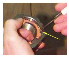
2. Place the blade of a flathead screwdriver in the slot located on the keeper leg.
