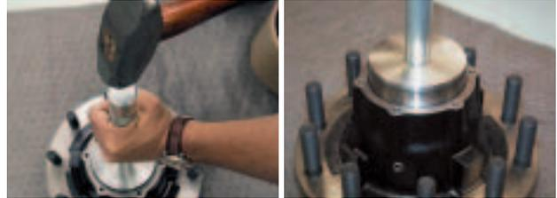
**Step 1** Thoroughly clean bearing cups and cones prior to installation.
