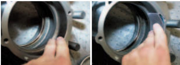
**Step 1** Inspect the hub bearing bores and shoulders for damage. The bores should be smooth and free from scoring, burrs, indications of cup spinning, or other forms of damage. Remove any burrs or raised areas using emery cloth, a file, or other appropriate tool.
