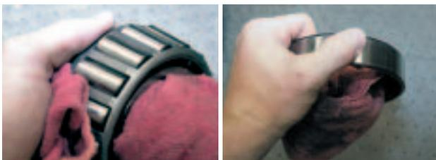
**Step 3** Inspect bearing cups and cones for damage. Bearings should be free from chips, contamination, and signs of excessive wear or excessive heat. Refer to bearing damage analysis literature for identifying possible bearing issues.
