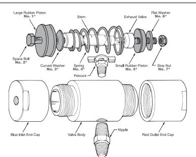
\*NOTE: Only the numbered parts (1-7) shown at left are in Repair Kit No. 900-1080.
