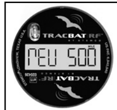
REV Mode shows RPM or RPK unit Programmed for.
