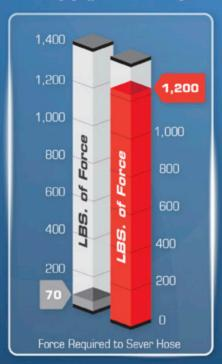
This test simulated a sharp metal object, forced upward between the duals, which can cut or damage the air hose.
