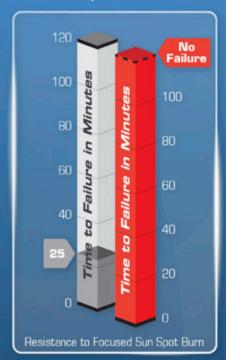
Aluminum wheels can concentrate sunlight into a beam that can reach temperatures of over 400° F which can cause hose failure or damage.
