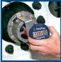
Install DataTrac Pro on wheel end.
