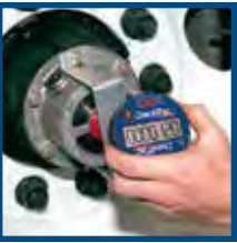
Install DataTrac Pro on wheel end.
