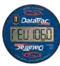
REV Mode shows RPM or RPK unit Programmed for.
