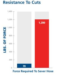
This test simulated a sharp metal object, forced upward between the duals, which can cut or damage the air hose.
