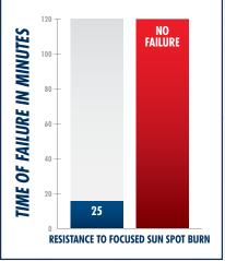
Aluminum wheels can concentrate sunlight into a beam that can reach temperatures of over 400° F which can cause hose failure or damage.
