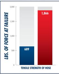
Tensile strength is important if the hose is snagged or stretched.
