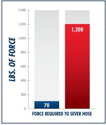
This test simulated a sharp metal object, forced upward between the duals, which can cut or damage the air hose.
