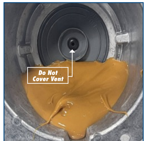
Figure 2: Fill Level for Semi-fluid Grease
