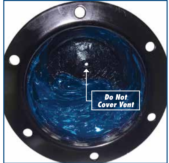
Figure 3: Wipe the inside of stamped steel hub cap with grease
