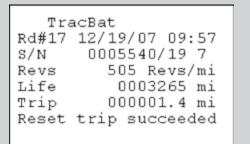
If you press the up ( $\uparrow$ ) arrow key, and the **HandBAT** does not succeed in resetting the trip, error messages will be given with the option to try again. When the trip is reset the reset is logged into memory for later download.
