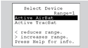
If you have an AirBAT sensor, use the up/down keys to highlight **Active AirBAT** from the **Select Device** screen.
