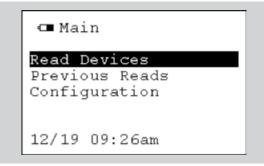
This screen is the Main Menu and is used as a selection screen for desired functions of the handheld reader. Select the function you wish to perform using the up ( $\uparrow$ ) or down ( $\downarrow$ ) arrow keys. You have three functions to choose from.
