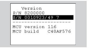
The version screen allows the user to tell which version and build numbers are currently programmed into the processors inside the unit.
