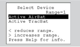
This is the primary screen option used to read your BAT RF tags installed on your vehicles. To activate this option press the up ( $\uparrow$ ) or down ( $\downarrow$ ) keys to highlight the appropriate option, then press the **Enter Key** found in the middle of the up/down and left/right arrow keys. After depressing the **Enter Key** you will be presented with the **Select Device** screen as shown below.
