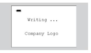
You will be returned to the previous screen with a notification of whether or not the **write was successful**. If the write to the AirBAT sensor works a screen similar to the one shown below will be displayed. The new limits should be shown on the screen.
