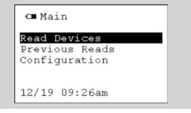
The battery indicator is in the upper left hand corner of the main screen (as shown above). It will show the current status of the battery. When the battery gets sufficiently depleted the unit will not allow the user to keep the device turned on. If a HandBAT becomes severely discharged the **HandBAT** will display a low battery message and then turn itself off automatically.
