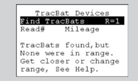
This may be caused by not holding your handheld reader within range of the TracBAT mileage sensor you wish to read. Please move to within the reading range and try again. If the problem persists, and you cannot read the desired sensor, then increase the range just a bit. Be careful not to increase range too much as you may begin to see sensors behind you instead of the sensor of interest. **See screen help for more info.**
