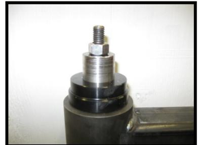
3. Place upper plate over upper mandrel and alignment bushing.
