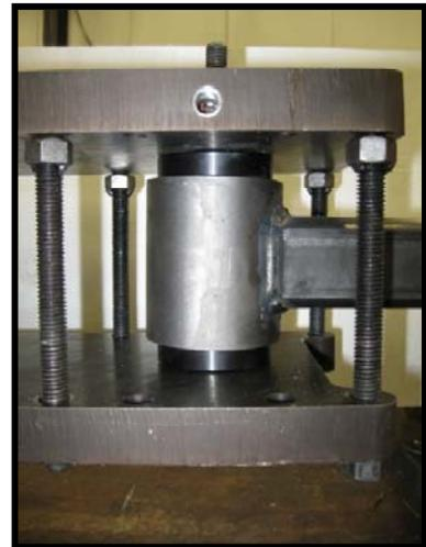
6. When these components are applied properly with the standard components, machining of the 5000 lbs GM axle is easily accomplished.
