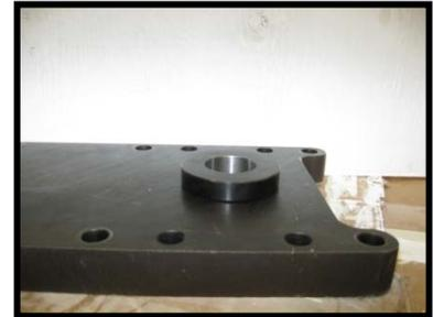
5. Place lower plate with special alignment bushing over lower mandrel, attach lower assembly to upper assembly using threaded rods and nuts. (Reference to standard instruction page 10 & 11)
