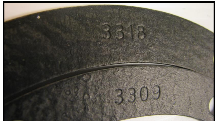
Figure 2 - Embossed part numbers on gaskets.
