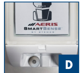
Example of using a pop rivet to install the bracket.
