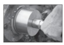
Tighten until the seal flange bottoms on the cage -or installation tool bottoms on cage (non-flange seals). Take care not to overtighten bolt/nut.
