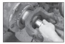
Step 6 Remove burrs and thoroughly clean yoke. Lube the seal ID. Install voke as shown.
